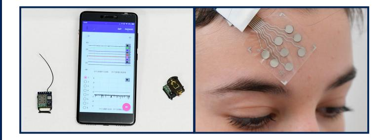
Wireless (BLE), wearable, up to 16-channel EEG/EMG biopotential,
