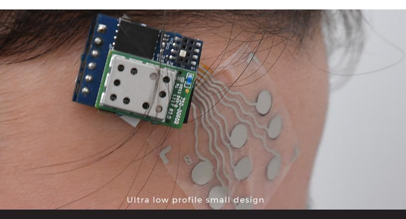
Can be hosted on any system that can access Bluetooth low energy: Windows, Linux, Android, iOS.
